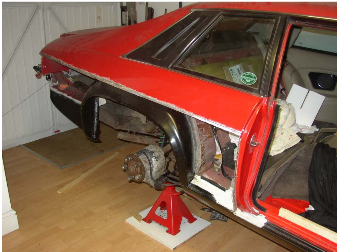
New inner arch fitted
