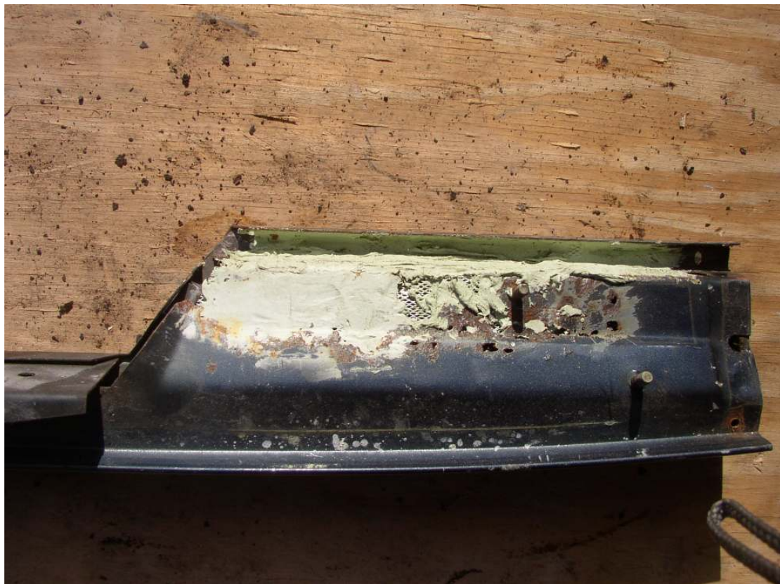
Boot plinth rust and boded repair
