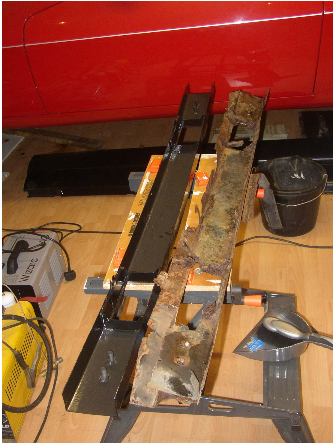
Bumper beam – new (left) and old (right)
